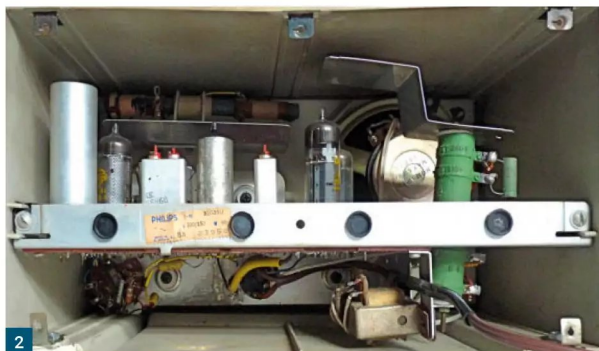
Fig. 1: Typical Philips AC/DC Radio of late 50s/early 60s. Fig. 2: Inside the back of the Philips AC/DC Radio. Fig. 3: Eddystone dropper resistor in parlous condition. Fig. 4: Eddystone 840A Power supply. Fig. 5: Barretter.
